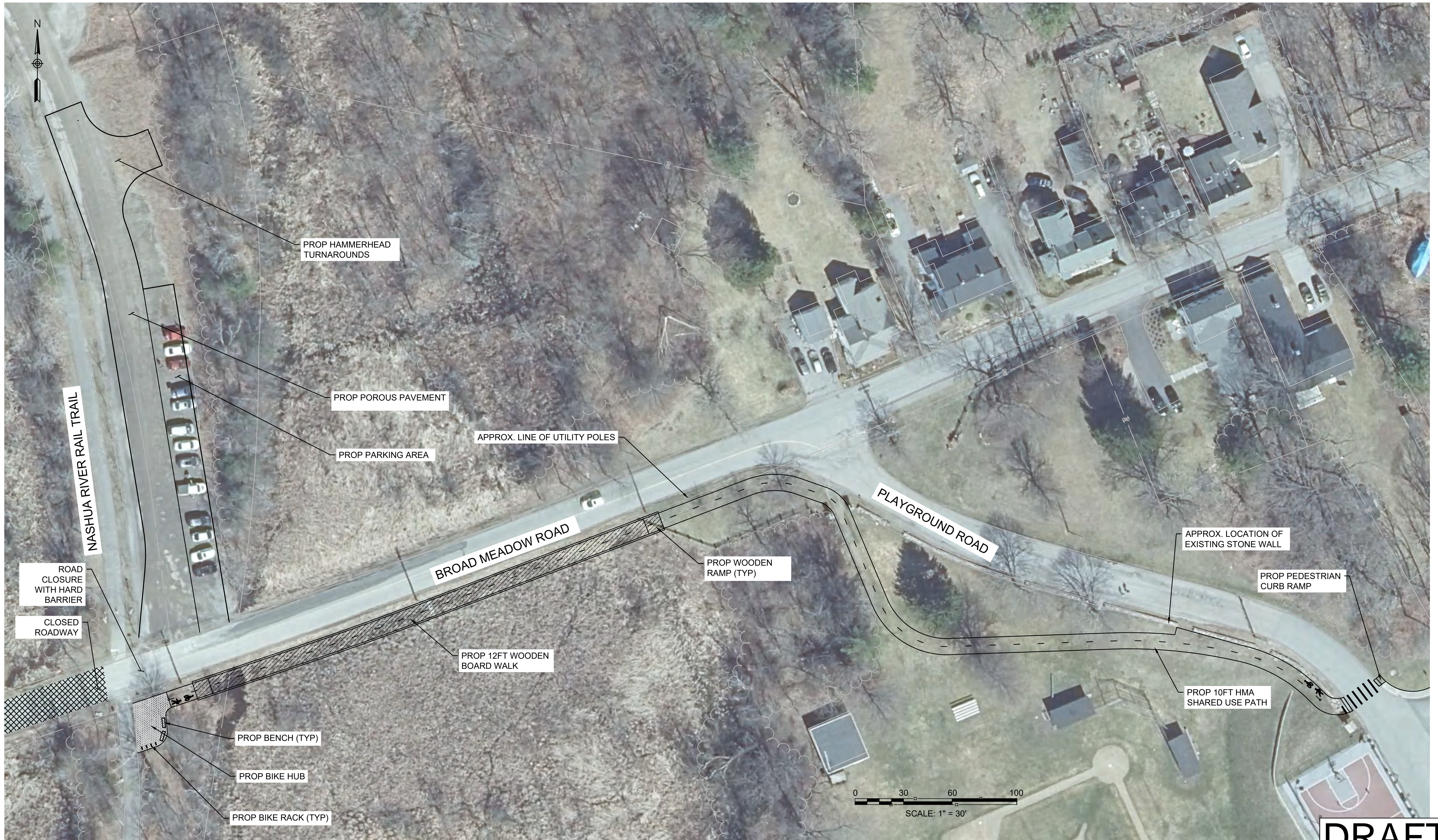
HOT MIX ASPHALT SHARED USE PATH ALONG PLAYGROUND ROAD WITH PEDESTRIAN/BICYCLE BOARD WALK ALONG BROAD MEADOW ROAD
